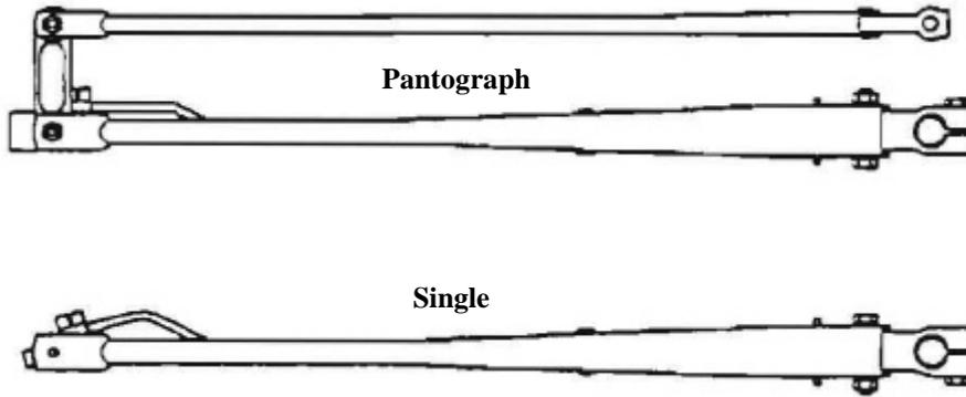
**2) Measure length on arm or main arm (if pantograph)**
